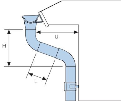
The measurement U is the projection of the offset. An SOKN one-piece offset is available with a fixed projection of 100mm.
